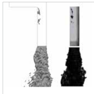
Fig. 1 - Internal nozzle flow test case . Left) developed LES-VOF solver; right) visualizations from experiments.
