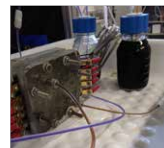
Fig. 3 - Vanadium Flow Battery device
