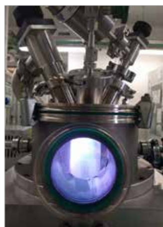
Fig. 1 - Plasma source (called NanoJeD) used for the fabrication
