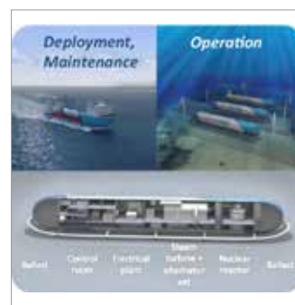
Fig.1 - Conceptual view of Flexblue power unit
