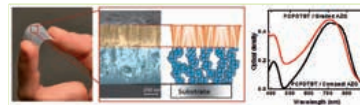
2. (left) A flexible transparent conducting scattering AZO layer on an ETFE substrate. (center) Cross-sectional SEM image and corresponding scheme of a graded AZO layer constituted by a compact conducting layer on a porous scattering layer. (right) Increase in optical density of a 30 nm PCPDTBT: the black curve shows the polymer absorption profile when it is deposited on a compact AZO layer, the red curve reports the absorption of an identical PCPDTBT layer grown on a graded AZO architecture.
