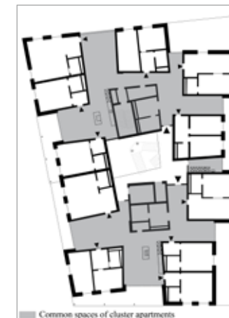
Fig. 1 – Layout of cluster apartments, building A, Mehr als Wohnen settlement, Zurich North, Scale 1:400 (Source: Own drawing based on architectural drawings of Duplex Architekten)
