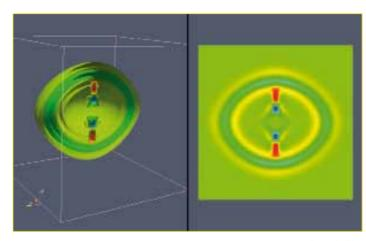
2. Seismic wave propagating in anisotropic medium. Pressure isosurfaces (left) and pressure on the yz plane (right). Artificial non-reflecting boundaries are applied.
