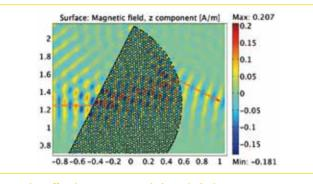
1. Superprism effect in nanostructured photonic device. Magnetic field, z component.
