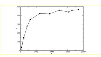
**1.** Speed up factor **S** of the parallel code versus the number of cells in physical space N for the driven cavity flow problem.  $S = T_{cou}/T_{cou}$  where  $T_{cou}$  and  $T_{cou}$  are the times used by the CPU and GPU respectively.
