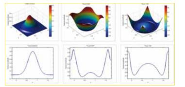
1. Numerical simulation of a seismic impulse in an isotropic medium with PML boundary conditions
