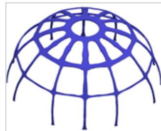
Fig. 1 - Topology optimized structure obtained via SIMPATY algorithm
