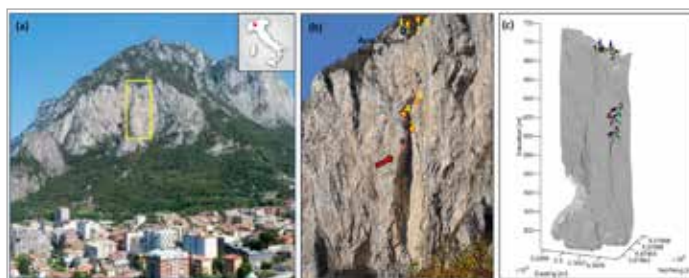
Fig. 1 - The study site in the southern part of Mount San Martino. (a) Front view of Mount San Martino from Lecco city. The yellow rectangle indicates the monitored area where the monitoring network was deployed. (b) Rock face with the positions of the five geophones and the acquisition board of the microseismic monitoring system. The red arrow indicates the partially detached pillar below geophone 4. (c) Photogrammetric model of the monitored area with the orientations of the five geophones.
