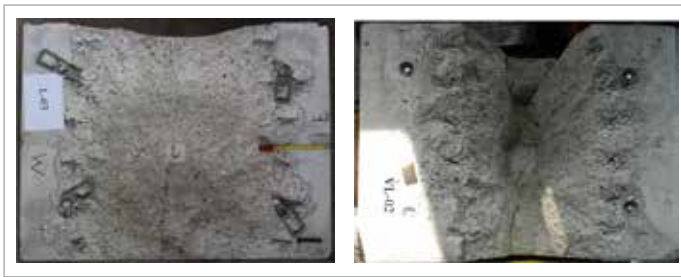
Fig. 1 - Two specimens after testing: (a) fastener with low bearing pressure and (b) fastener with very low bearing pressure.
