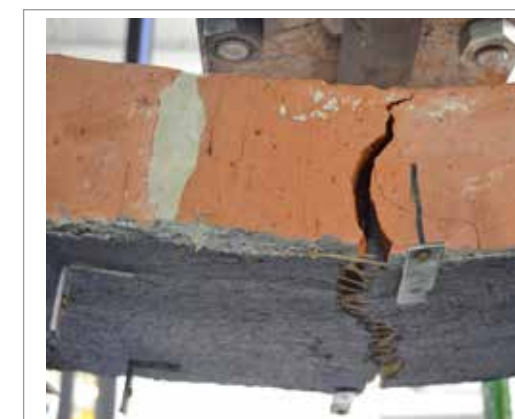
3. Bending test: failure mode
