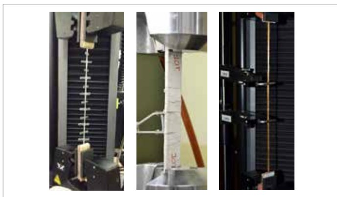
1. Tensile tests on dry yarn and FRCM system
