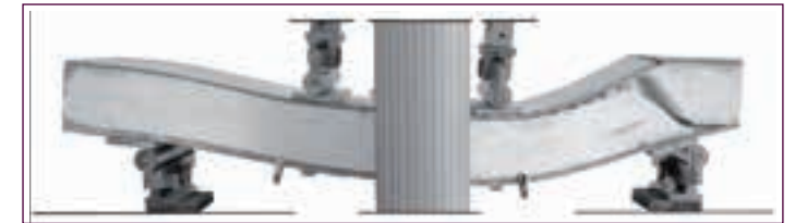
1. Four point load test on big sandwich beam.
