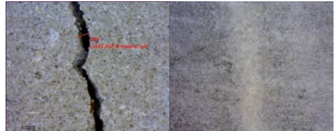
2. Healed crack for specimen (a) pre-cracked up to 150 µm; (b) 6 months of water immersion
