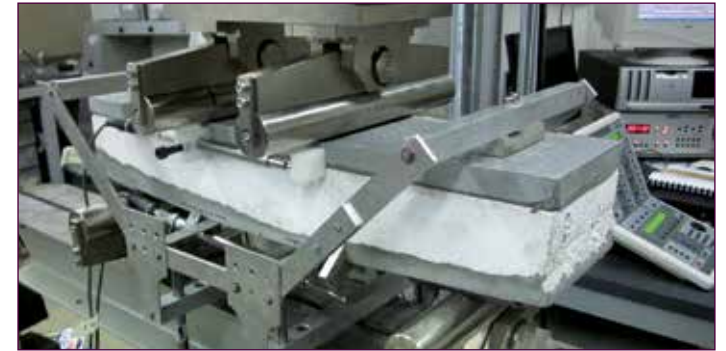
1. Four point bending test on a sandwich specimen
