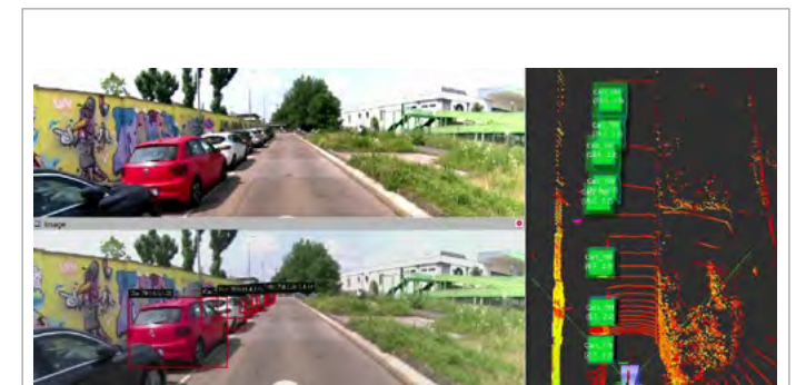
Fig. 3 - Real-time obstacle detection using vision-radar sensor fusion.
