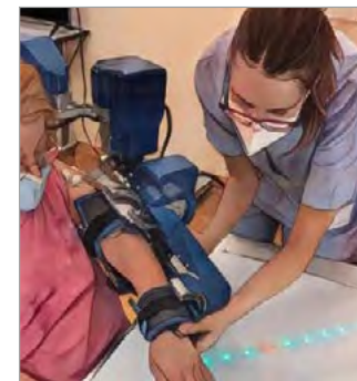
Fig. 2 - Therapist-robot interactions: the therapist manipulates the robotic system to teach trajectories and support profiles to support the patient during the therapy.
