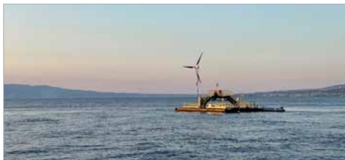
Fig. 1 - Picture of the 1:15 prototype deployed in the test site at NOEL (Reggio Calabria, IT) for a 1-year test campaign.
