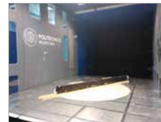
Fig. 2 - Wind tunnel test of a conventional train.
