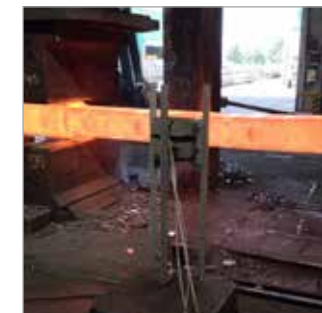
Fig. 2 - Laser scanner device measuring the section of a prismatic forging bar
