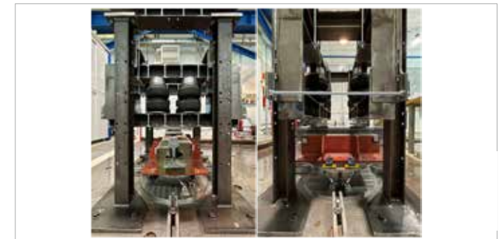
Fig. 2 - Purposely developed laboratory test rig to determine dynamic properties of the Embedded Rail System.
