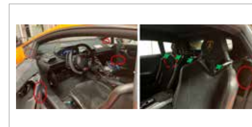
Fig. 2 - Sensors and actuators of the active control system used to equalise the sound field.
