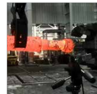
Fig. 3 - Camera device measuring the geometry of a cylindrical bar
