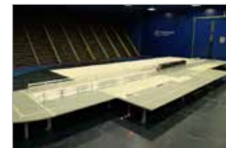
Fig. 3 - Wind tunnel test of a high-speed train in presence of windbreaks.
