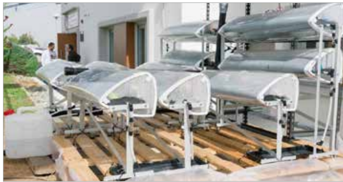
Fig. 1 - Modular desalination system inspired by Mangrove Ecosystem
