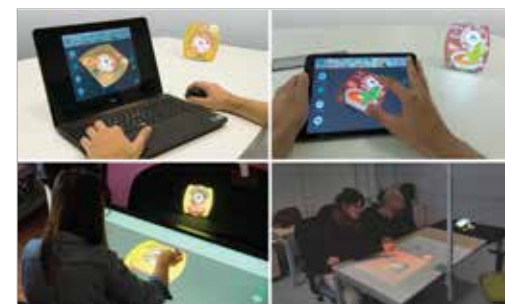
Fig. 2 - Representation of the 4 different types of interfaces (desktop, tablet, touch screen and tangible interface) developed to support the use of the SAR platform according with the design scenario.
