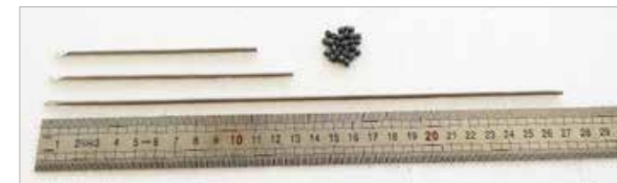
Fig. 2 - The feedstock used for extrusion and bi-lumen needles fabricated by feedstock extrusion processing
