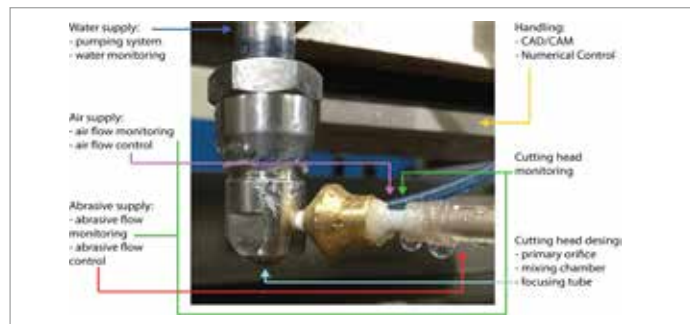
Fig. 1 - The \mu AWJ cutting head (left) and the injector (right).
