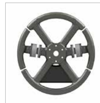
Fig. 2 - Instrumented Steering Wheel
