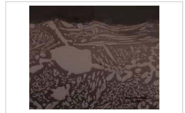
Fig. 2 - SDSS after controlled shot peening
