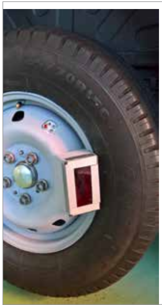
Fig. 3 - Wheel Force sensor prototype
