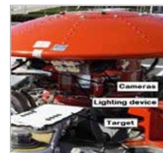
Fig. 1 - The measurement system integrated with helicopter main rotor
