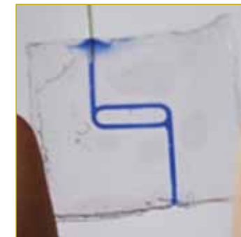
3. Image of closed devices with good sealing. The liquid remains just inside the channels and clearly outlines the microchannels pattern.
