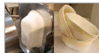
Fig.2 – Press-forming process and paperboard trays.
