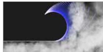
Fig. 1 - A humidity-responsive self-actuator.
