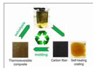
Fig. 1 - Recycling scheme of a composite based on a reversible polymer network. Solvolysis allows for the efficient separation of both reusable fiber and resin component.
