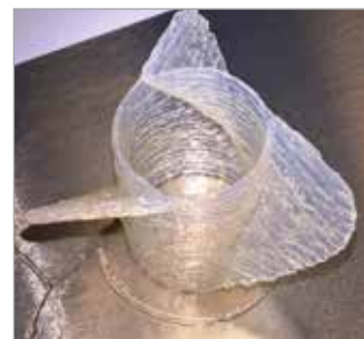
Fig. 1 - 3D printed propeller with the formulation at 5% of short glass fibres
