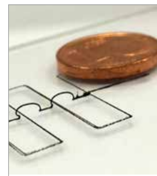
Fig. 2 - optical photograph of a ldm-based 3d printed conductive filament deposited in a freeform manner (a 1 cent euro coin is reported in the image for dimensional reference)
