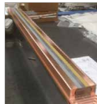
Fig. 2 - aw of the low impedance secondary collimator prototype for HL-LHC, delivered at CERN in November 2016. It features a Mo-Gr bulk in 3 configurations: without coating, with Mo layer and with TiN layer
