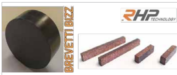
Fig. 1 - Left: plate of Mo-Gr (Brevetti Bizz, Italy). Right: bar samples of Cu-CD (RHP Technology, Austria)
