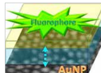
2. Schematic illustration of Multilayer structure for the generation of MEF.
