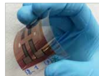
2. PSC devices produced on flexible substrate by all solution R2R-compatible processes.
