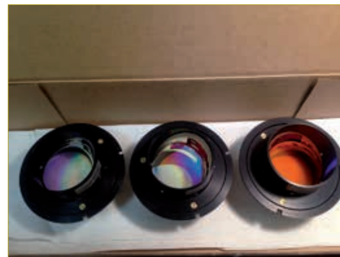
2. Astronomical dispersive elements designed and produced for the ALFOSC spectrograph at La Palma (ES)
