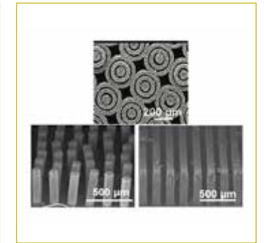
2. SEM images of micro-structured VACNT forests: (top) concentric rings, (bottom-left) pillars and (bottom-right) lines.
