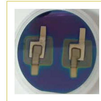
2. Top view image of two Thin-solid film Li-ion microbattery prototypes deposited over a Si/ \text{SiO}_2 wafer.
