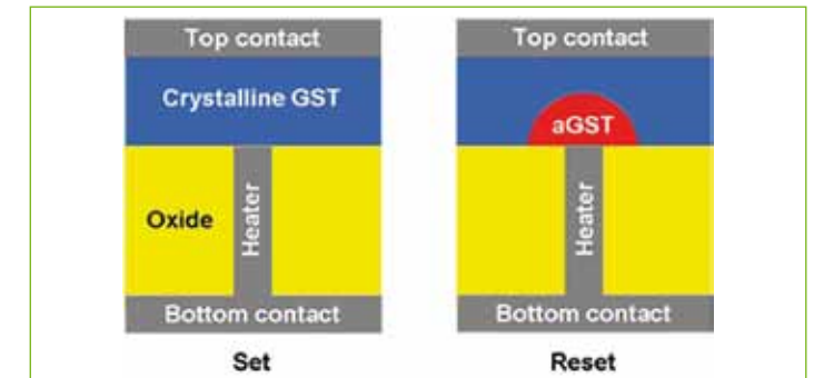
1. Schematic of a simple cylindrical PCM. The active chalcogenide material is contacted by a thin metallic plug, the heater, which heats the GST through electrical pulses. The cell is in the set state when the chalcogenide is all crystalline (left), by contrast the reset state (right) is characterized by the presence of amorphous chalcogenide
