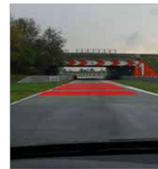
Fig. 2 - Braking point AR information projected outside the vehicle.
