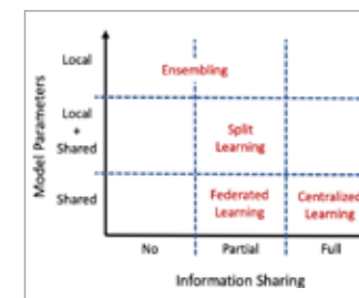
Fig. 2 - Overview of distributed learning paradigms, classified in our framework by degree of Information Sharing and Model Parameter displacement between the distributed models.
