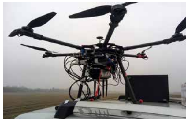
Fig. 1 DoA estimation prototype fitted to a Tarot X6 UAV with a 2x2 2.4GHz beamforming array fitted to the bottom.
