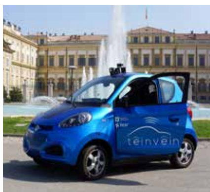
Fig. 1 Image of the experimental vehicle. It is possible to notice the Lidar and cameras sensors mounted on the roof and the two GPS sensors on the front and the rear of the car
