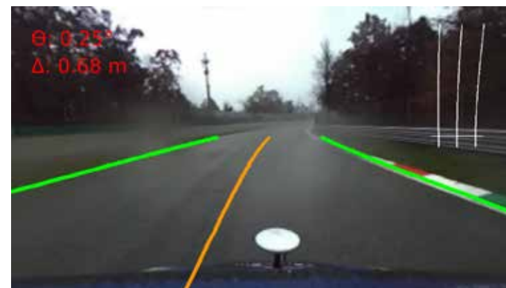
Fig. 2 output of the lateral line detection pipeline. In green are represented the detected lateral lines; in orange, the road centerline; in red, the computed ego-vehicle heading and lateral offset. In white, on the right, the bird-eye view projection of the lines.
