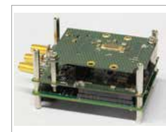
Fig. 3 - General purpose SPAD camera assembly (without housing). The topmost board hosts the detector, the middle board provides all power and interfaces, while on the bottom one is an FPGA board.
