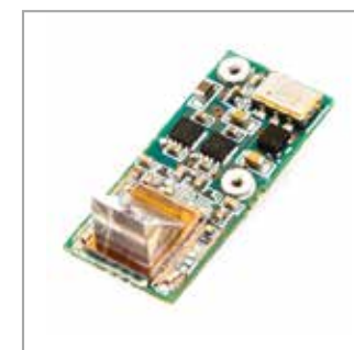
Fig. 3 - Photograph of circuit board with bonded digital SiPM IC and prism mounted on top for the SOLUS optode.
