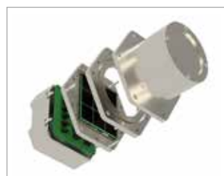
Fig. 1 - Developed spectrometer enclosure. The cylindric shape is designed to contain the crystal, the hexagonal flange allows the exploitation of the system in laboratory setups and the upper box hosts the electronics.
