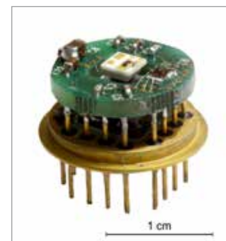
2. Compact InGaAs/InP SPAD System-in-Package, which integrates detector, cooler and front-end electronics in a TO-8 can.
