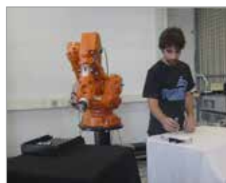
1. ABB IRB 140 industrial robot performing a pick and place task in a dynamic environment populated by humans. The proposed control algorithm enhances human safety by exploiting sensors measurements
