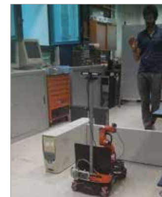
2. a KUKA youBot interacting with a human operator in an unknown environment. The robot is controlled through the proposed Model Predictive Control strategy
