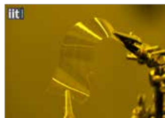
1. A Fully-printed electronic circuit. Techniques employed for this sample fabrication are ink-jet printing and bar-coating
