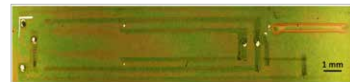
3. Optical micrograph of the fully inkjet printed dusk sensor comprising organic Schmitt trigger and planar organic photodetector.
