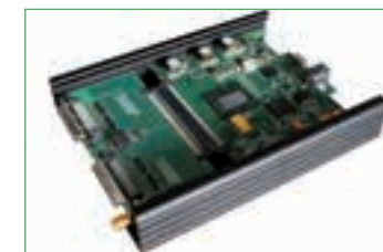
2. 64-channel cross-correlator module
