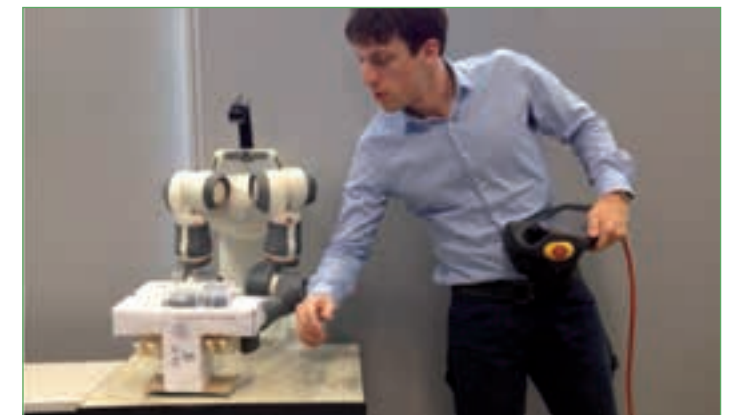
3. The second collision avoidance strategy is applied on a dual arm task.
