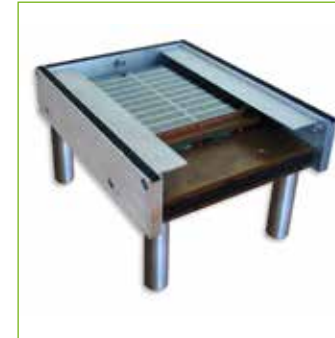
1. HICAM 10\times 10 has a global FOV of 12\times 10\text{cm}^2 , using 100 SDDs, aligned in a 10\times 10 matrix. The fundamental unit of both systems is a single square SDD has an active area of 1\times 1\text{cm}^2
