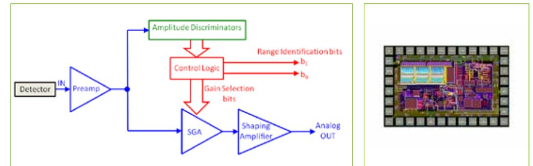
1. Simplified blocks schematic of the designed front-end for photodiodes – single channel version. The different colors identify different ASIC sections: analog (blue), digital (red) and mixed-signal (green).
