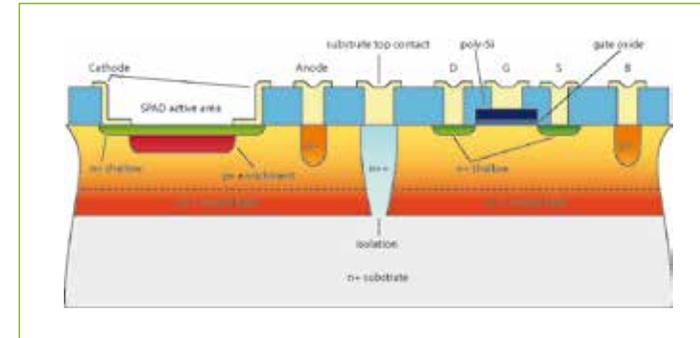
1. Cross section of a custom SPAD and of a nMOS fabricated by the same technology.
