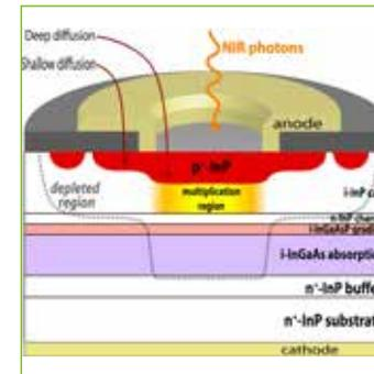
1. Structure of a planar front-illuminated InGaAs/InP SPAD.
