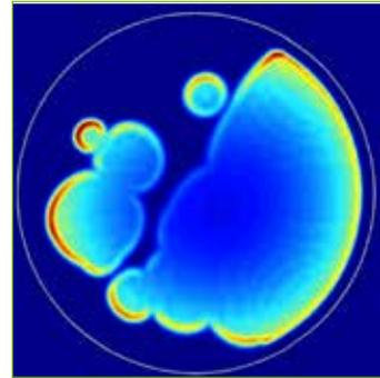
**1. Carrier distribution, 700ps after injection, simulated with the 2D avalanche spread simulator. It is worth nothing the secondary injections, due to photon-assisted propagation, which dramatically affect the avalanche propagation.**
