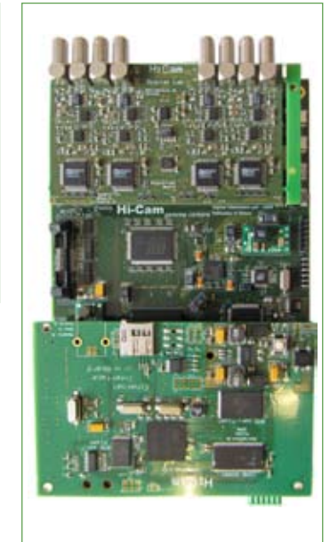
3. Multi-channel processor for medical imaging purpose
