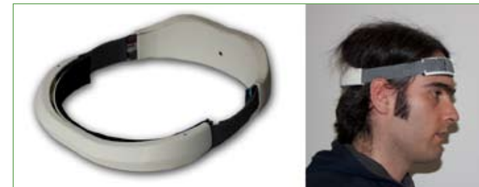
2. Wearable device developed during our research. It acquires BVP, GSR and a 3-axes accelerometer with bluetooth data transmission
