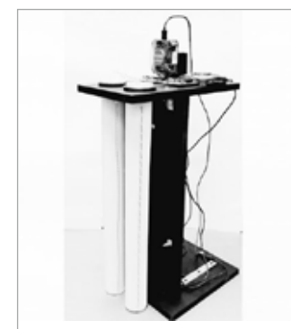
Fig. 2 - The proposed level measurement system based on phase-shift considering different two-conductor waveguides
