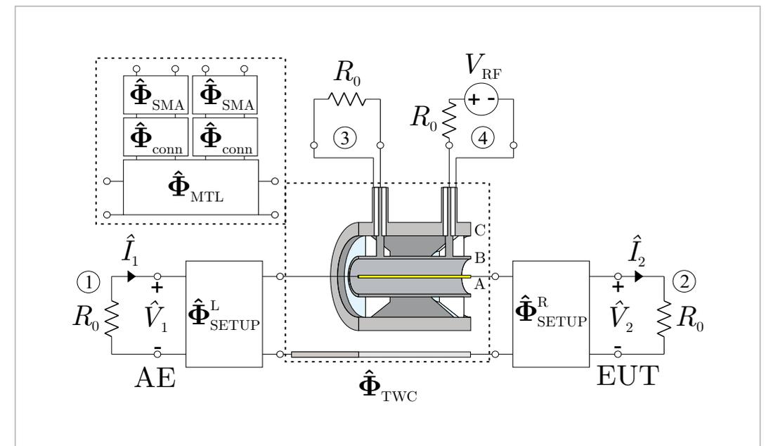
Fig. 3 - Distributed-parameter model of the TWC mounted on the CF. The TWC model is detailed in the up-left panel.
