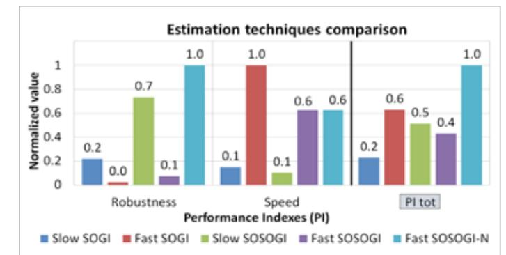
Fig. 3 - Normalized comparison of the angular quantities estimators in terms of robustness and fastness. A global combined normalized index is reported in PI tot.
