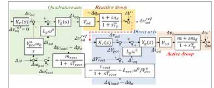
Fig. 2 - Dynamical model of the converter under droop regulation.
