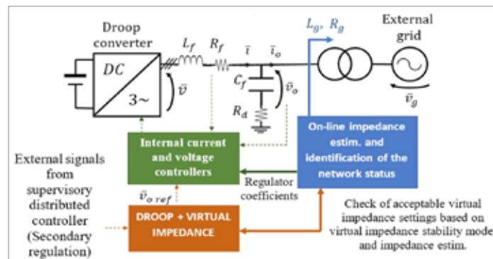
Fig. 1 - Enhanced-droop architecture: each sub-control is designed in order to guarantee the system stability. The dynamical effects of each sub-control in the converter stabilization both in grid-connected and island mode are analysed.
