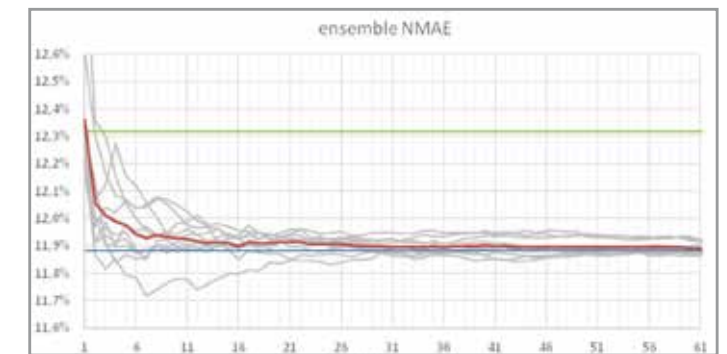
2. NMAE of ten random ensembles (grey lines) as a function of the size of the ensemble basin (number of trials). The ANN has 120 neurons and the Levenberg-Marquardt training algorithm. The mean NMAE of the ensemble forecasts is in red, the mean NMAE of one thousands forecasts is the upper constant green line and the ensemble NMAE of one thousands trials is the lower constant blue line.
