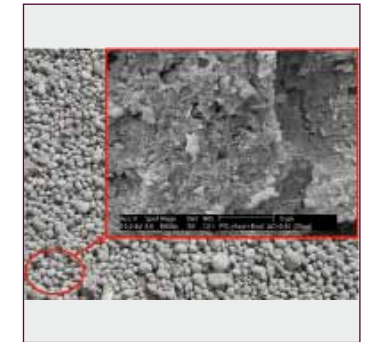
1. Granular materials after thermal desorption step, with an enlargement at microscopic scale (by scanning electron microscope)
