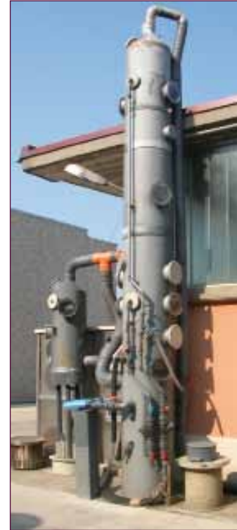
1. VOCs removal from gaseous emissions. Pilot-plant experiments on biotrickling filters and rotating biological contactors
