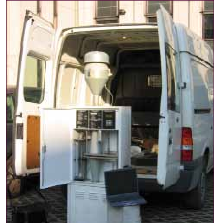
2. Mobile Lab for air quality monitoring
