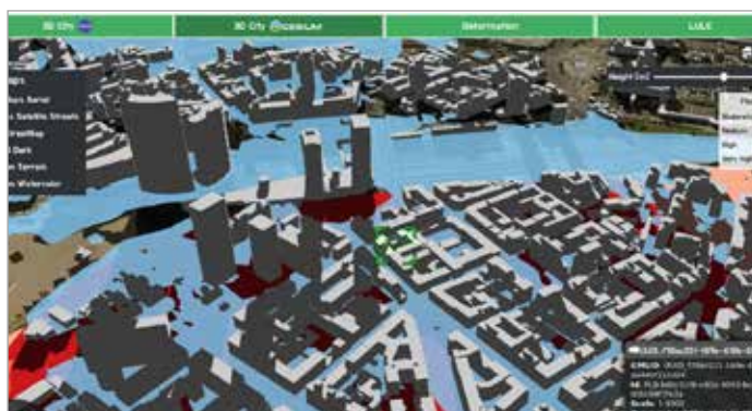
Fig. 1 - Flood simulation in Milan with a flood risk map and the visualization of CityGML data on a virtual globe created using CesiumJS
