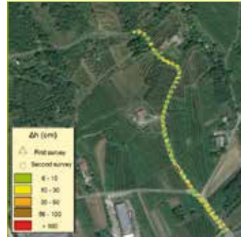
1. Differences between the LiDAR PST-A DTM and some RTK GNSS points surveyed in the Adda River Valley.
