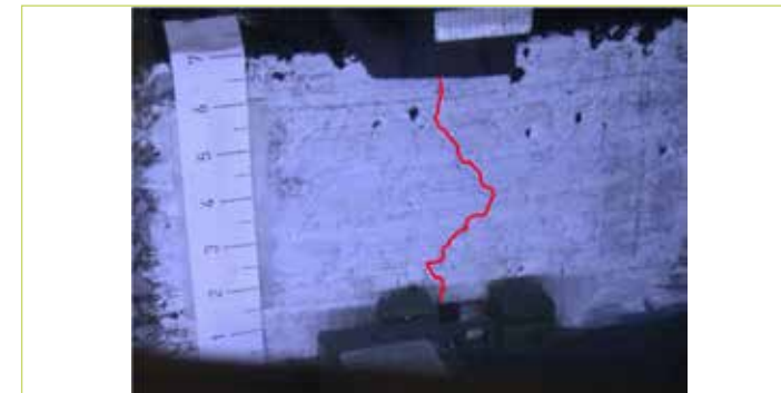
3. Crack path in reinforced double-layered system.
