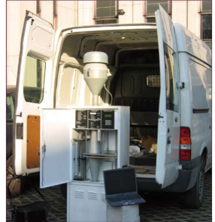
2. Mobile Lab for air quality monitoring
