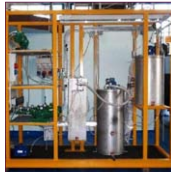
1. Picture of the anoxic-aerobic pilot MBR
