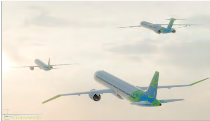
Fig. 1 - Rendering of the three configurations considered inside the U-HARWARD project: the folding wing tip configuration in the foreground, the strut-braced wing configuration on the top right corner, and the traditional configuration with a higher aspect ratio on the left.
