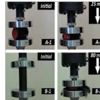
Fig. 2 - Crushing of hexachiral filled composites in A) lateral B) uniaxial direction
