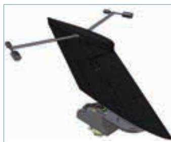
1. T-tail aeroelastically scaled wind tunnel model.
