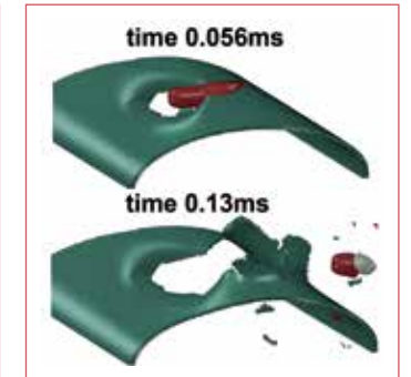
3. Numerical reproduction of the ballistic impact on the aluminum shaft at two different instants
