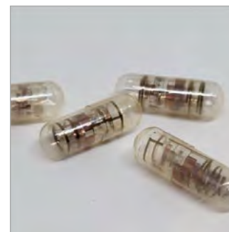
Fig.2 - Demonstrative picture of the connection between a fully printed edible logic circuit and an edible rechargeable battery.
