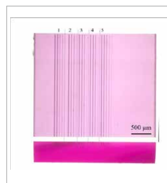
Fig.1 - Optical microscope image of the waveguide integrated quantum sensor in the DNV-diamond sample from overhead (top) and cross-section (bottom) point of view.
