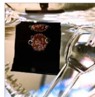
Fig. 1 - Picture of an HPC in the electrochemical cell. On its surface, H_2 bubbles can be observed.
